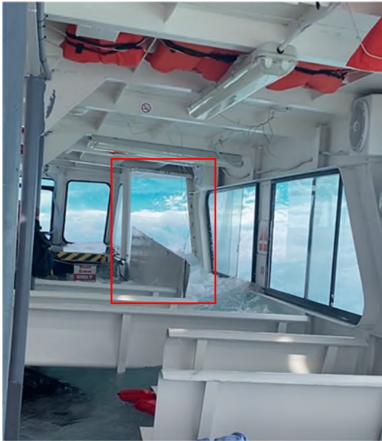
Focus Point 2: Lightweight door fitted on Islander III being dislodged (Source: shared by member of public)
