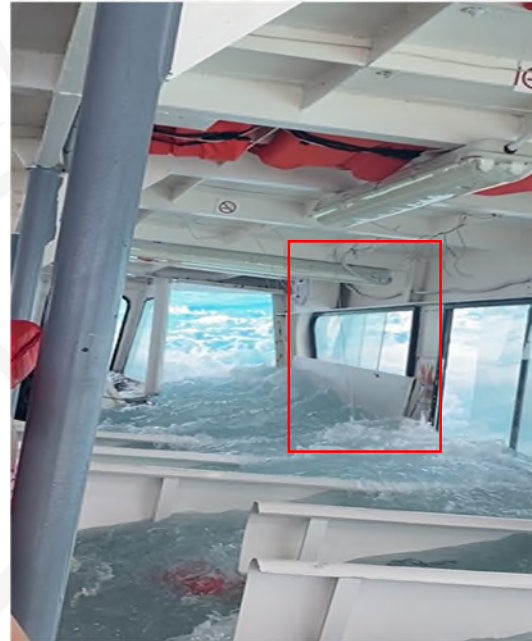
Focus Point 2: Lightweight door fitted on Islander III being dislodged (Source: shared by member of public)
