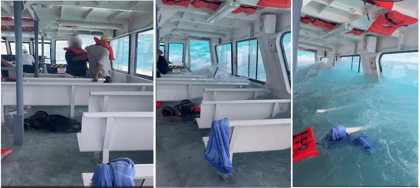
Images of initial water ingress, leading to progressive flooding after power increase (Source: shared by member of public)
