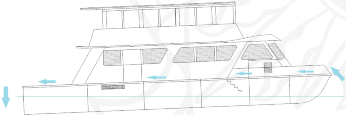
Boat master’s mental model of Islander III trim for water flow
