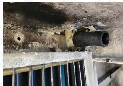
Focus Point 1: Refloated hull of Islander III. Left: Bathroom vent and gooseneck vent. Right: Gooseneck vent without flooding protection
