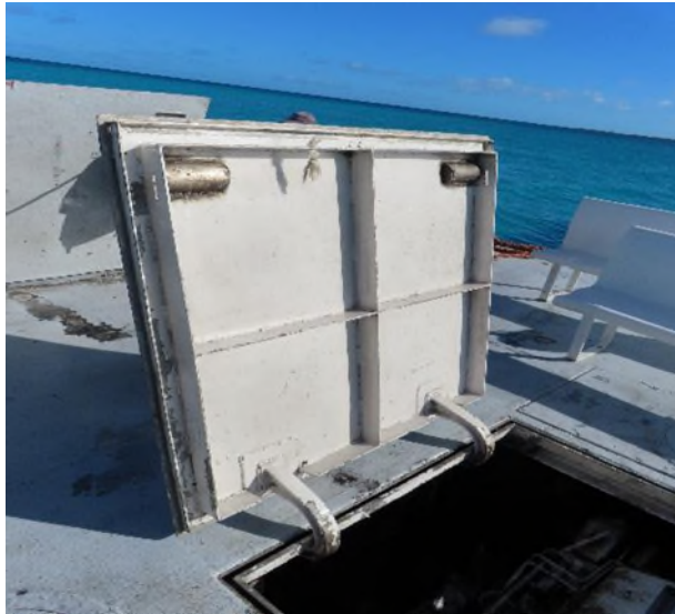
Engine room hatch - no dogs or gasket. Air intake without flooding protection
