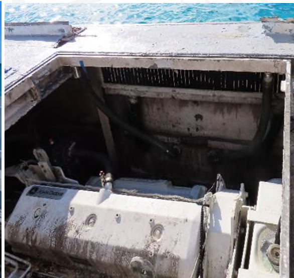
Engine room hatch - no dogs or gasket. Air intake without flooding protection
