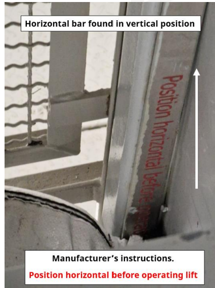
Figure 7. Horizontal bar found in vertical position.
